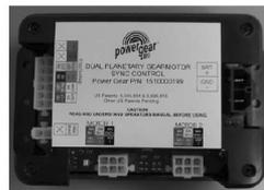
Fig.1 Slideout Controller
