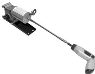
4. If the cables tighten, and the motor is difficult to turn, **REVERSE THE DIRECTION. OVERTORQUEING CAN HAPPEN, RESULTING IN SEVERE DAMAGE.**
