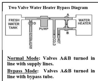
**NOTE:** In the diagram: Valve A is the black valve, valve B is the white valve. Valve D is the suction (siphon) valve that has the clear hose attached to it for siphoning in antifreeze, sanitizer or fresh water from an external container. This valve is typically located at the water pump.
