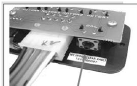
Figure 2 Set Stops/Clear Fault Button
