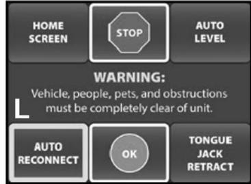
5. The system will retract all stabilizer jacks and the rear leveling jacks, then extend or retract the tongue jack until proper connection height is achieved. Display will read “Auto Reconnect in Progress”. (M below)
