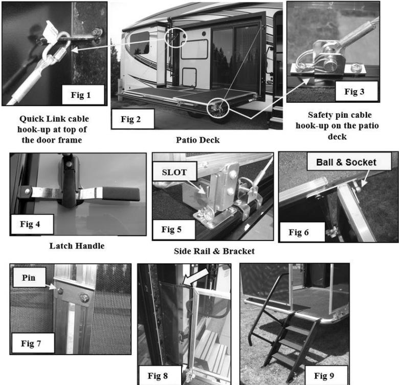
To set up the patio deck, unlatch the two keyed handles from the side of the RV (Fig 4). Lower the patio deck until the cables on each side support it. Support cables are attached at the top of the door opening with a quick link (Fig 1) and to the deck with a safety pin (Fig 3).
