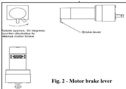
Fig. 2 - Motor brake lever
