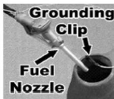
Fuel Nozzle in contact with receiving tank
