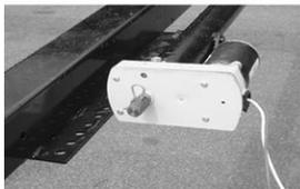
Fig. 3-Hex Head Crank Extension
