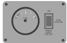
Single Tank Fuel Gauge & Selector Switch
