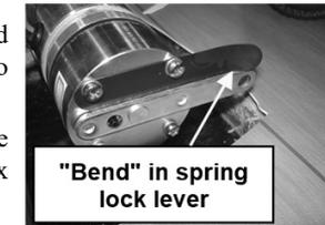
**DO NOT** remove boot. Removal of rubber boot will void manufacturer's warranty. Rubber boot removed from end of motor only to show brake lever and spring lock.
