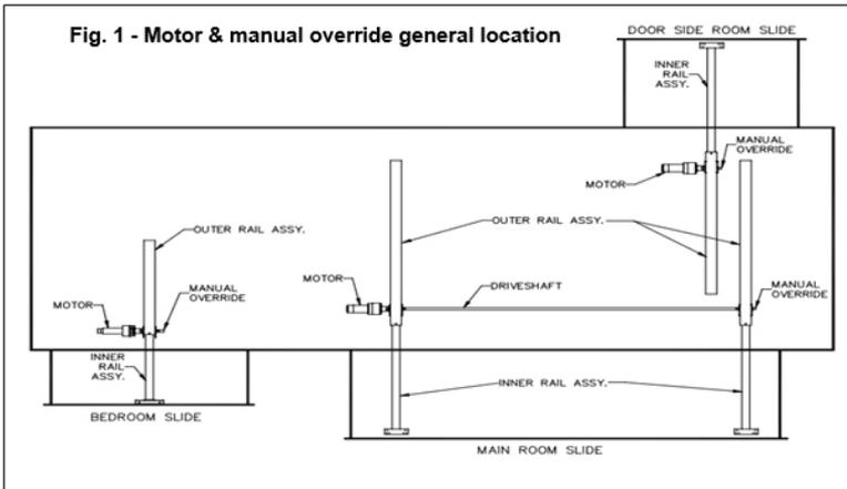
6. The room is now free to move. Using either a 5/8" or 3/4" wrench or socket, crank the room either in or out completely. If the slideout system is supplied with a gearbox override (optional), use the crank handle to move the room.
